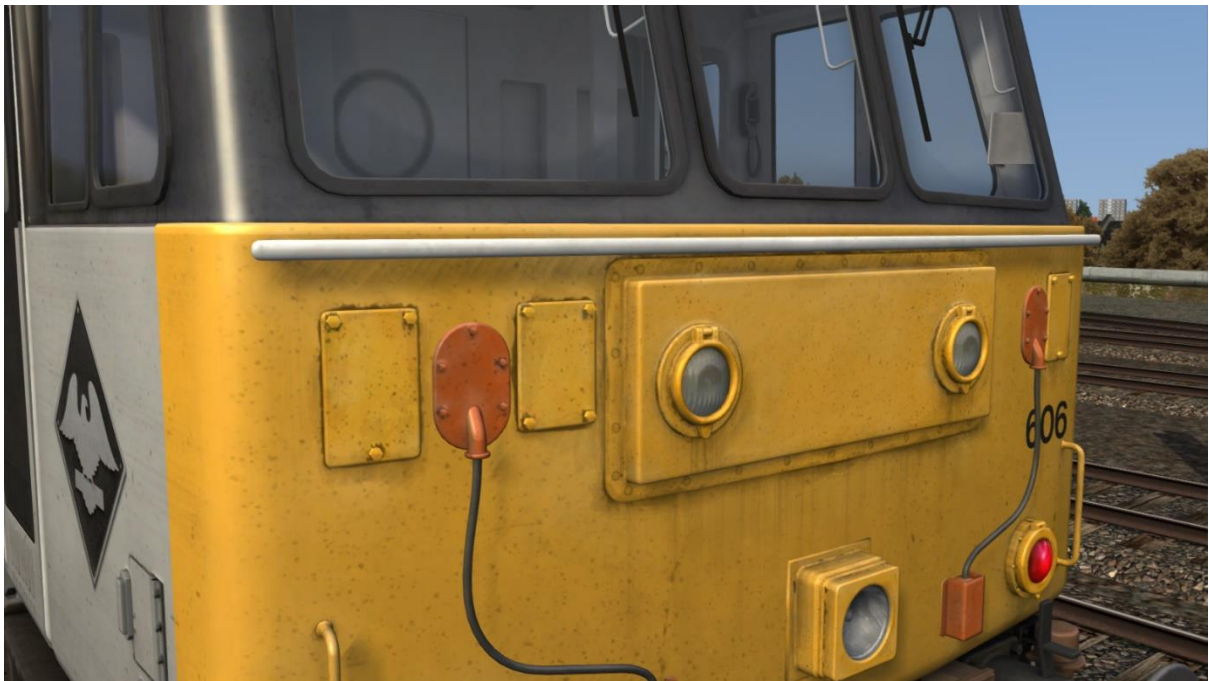
Plated over original multiple working jumpers
