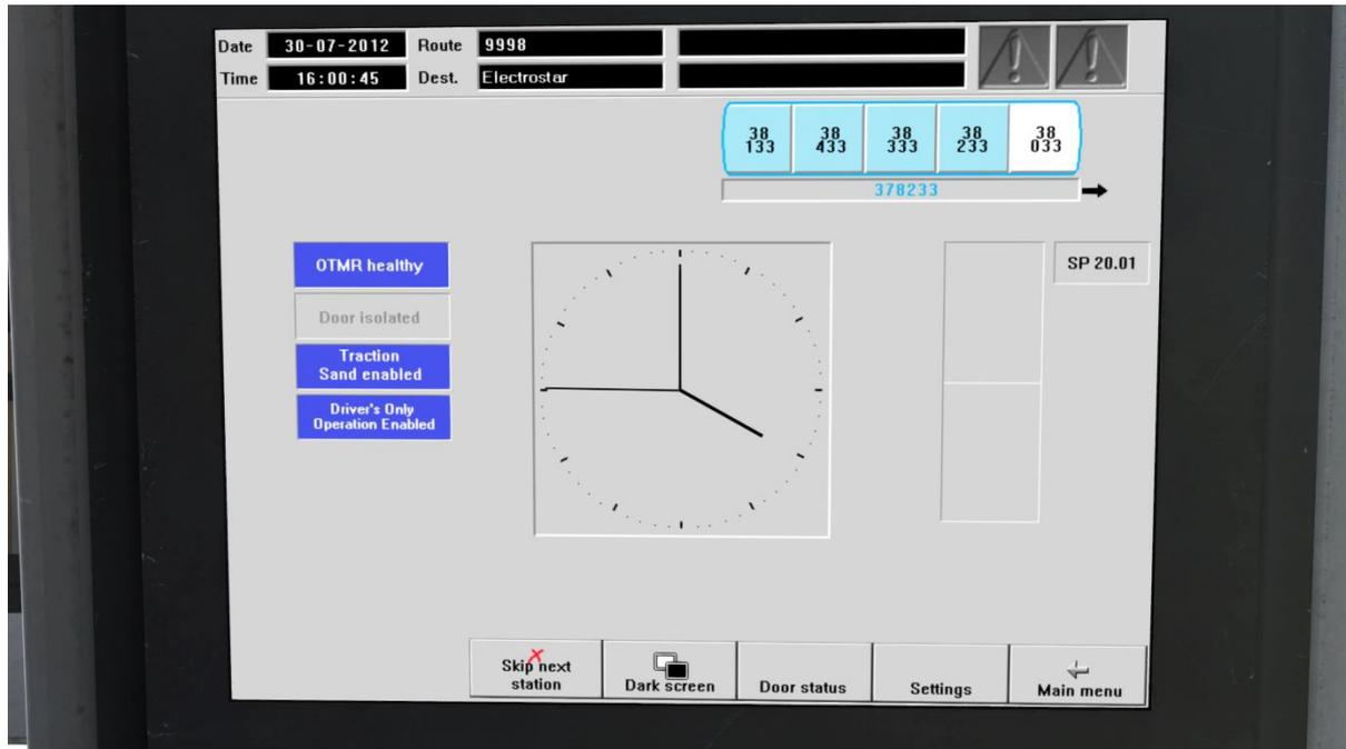
This screen shows the status of the On-Train Monitoring Recorder (OTMR), door isolations, traction sand and Driver's Only Operation (DOO). Out of these four things, only the 'Driver's Only Operation Enabled' indicator is dynamic. The other three are static as their state changes have not been simulated in this pack.
