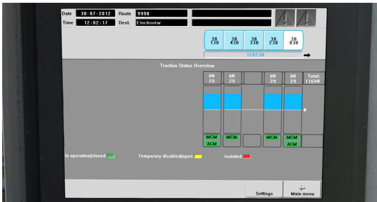
This screen shows the tractive effort being provided by each pair of traction motors on your train whilst accelerating or braking. It also shows the status of each Motor Converter Module (MCM) & Auxiliary Converter Module (ACM). The MCM is vital to the operation of the traction motors and the ACM powers vital systems on the train.
