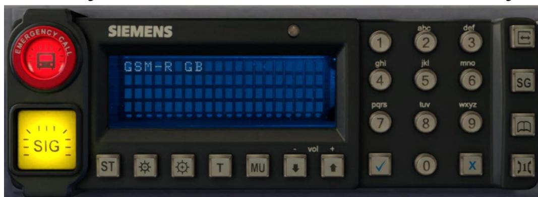
Beginning in 2013 and completed by 2016, Global System for Mobile Communication - Railway, more commonly known as GSM-R, replaced the existing National Radio Network (NRN) & Cab Secure Radio (CSR) systems. This communication system and its accompanying unit has been simulated to the best of our ability within the simulator. Please see below for how to register & deregister your train:
