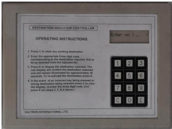
A fully functioning electronic destination display is provided with both the old triangle-based and new dot matrix variants represented. Instructions on how to operate the display can be found on the 'Vultron' destination indicator controller in the cab (pictured left). For each livery, a set of relevant destinations are provided. Please see below for a list of
